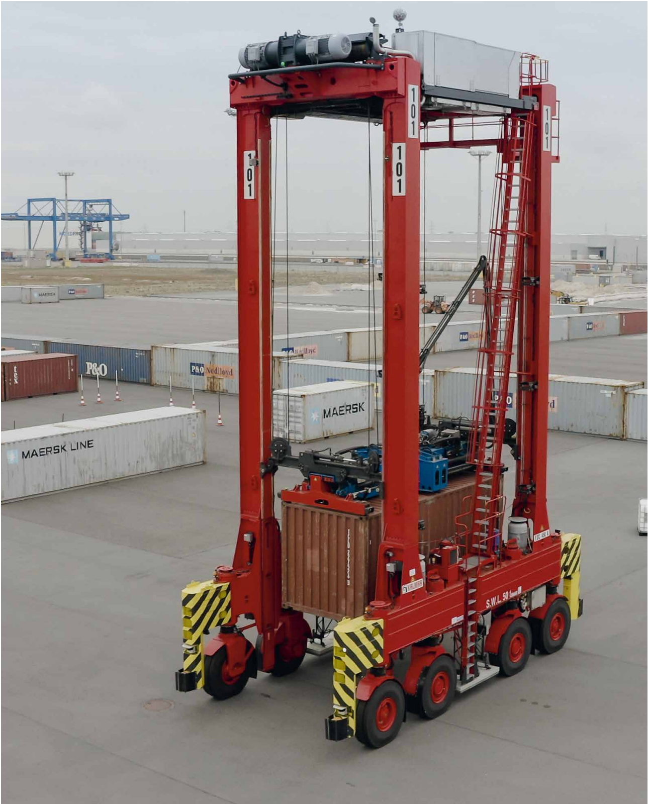
Driverless straddle carrier deployed on the STRADegy automation project in Wilhelmshaven.
